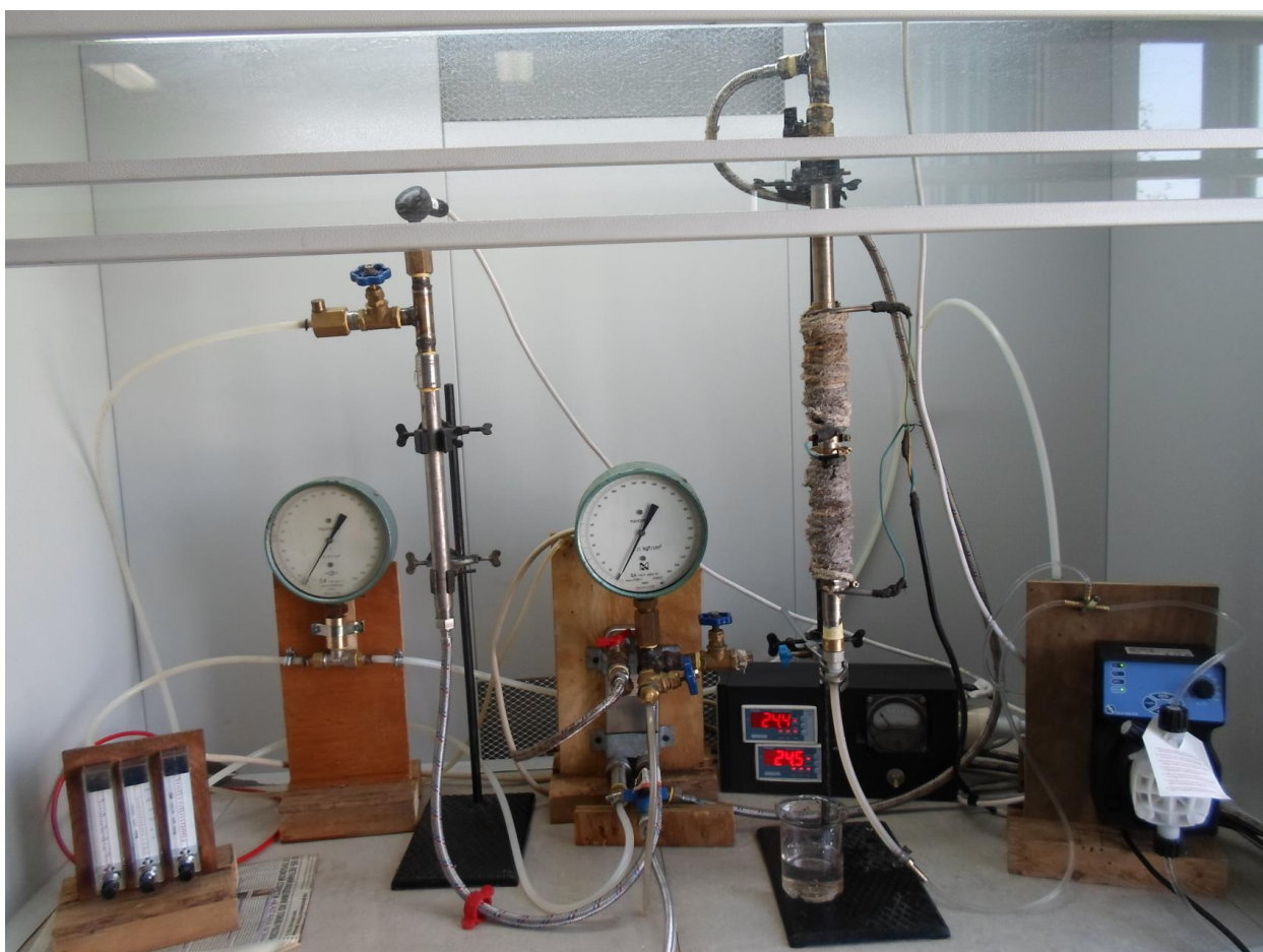
Figure – Laboratory installation of a 2-zone filter reactor for phenol oxidation
